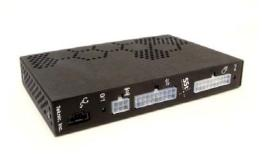
Servo controlling torque requires synchronized control of all motor phases with respect to the magnetic field of the motor's rotor. Conventional torque amps control each motor phase with a separate, dissociated current loop servo. This scheme ignores the fact that the motor phases are tied together and thus interdependent. Furthermore, small errors in each phase can combine to create a large vector (torque) error.
