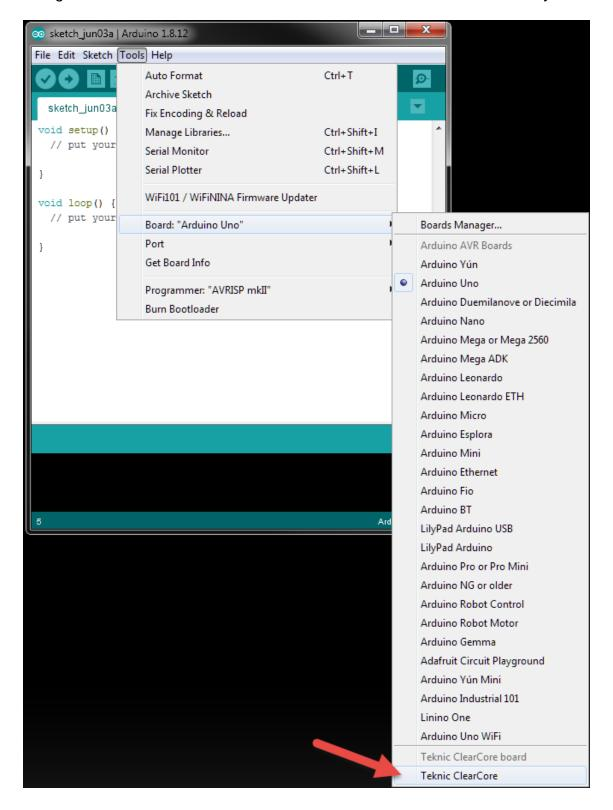
6) Supply power to your ClearCore (see <u>ClearCore User Manual</u> for detailed power information) and connect the ClearCore to your PC using a USB cable. Once connected, select Tools > Ports. Select the port named "Teknic ClearCore", e.g. "COM 11 (Teknic ClearCore)". Your COM port number may be different.
