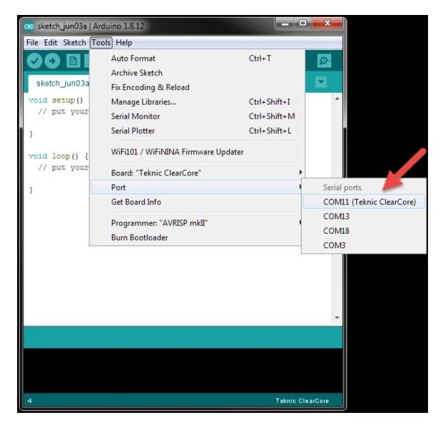
7) You can now upload a sketch to the ClearCore. To quickly verify that you can upload a sketch, select and upload one of the ClearCore example sketches included in the ClearCore Arduino Wrapper package, under File > Examples > Examples for Teknic ClearCore.
