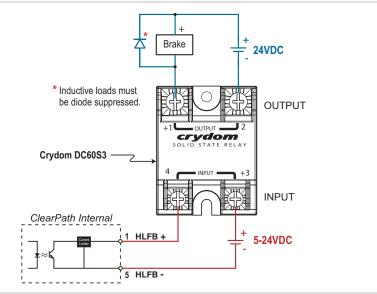
HLFB circuit controlling an SSR / brake setup
