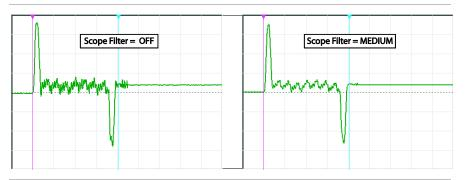
Effect of Scope Filter on trace display
