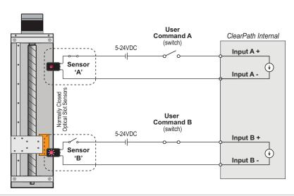
Move to Sensor: Inputs and Timing Diagram with example application sketch
