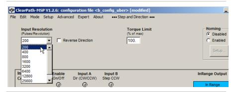
With the above Input Resolution setting, it takes only 200 step pulses to make this [800 count] motor rotate one full revolution.
