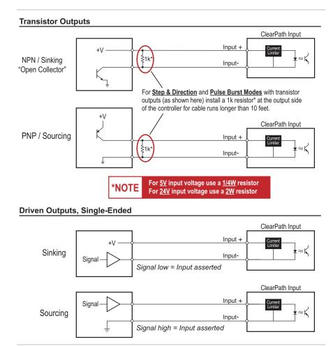
Interfacing digital outputs to ClearPath Inputs
