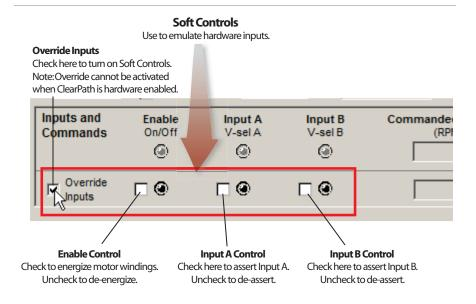
Check "Override Inputs" box to turn on Soft Controls
