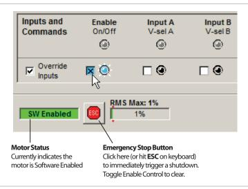
Enable ClearPath using Soft Controls
