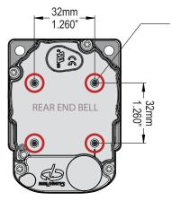
Mounting Boss (4 places) Inner dia: 0.125" (3.17mm) Use #6 or M3.5 thread cutters. Max penetration into boss: 0.28"
