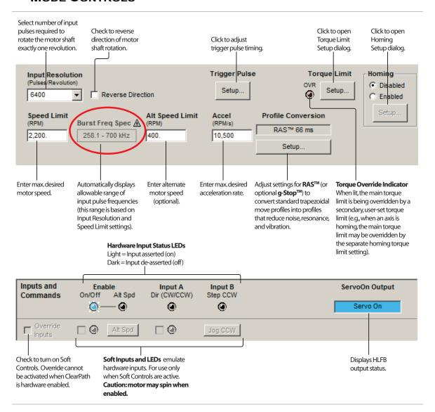
**Note: Input Resolution** (see upper left of mode controls screen capture above) is defined as the number of pulses that must be sent to the motor's input (Input B in this mode) to make the shaft rotate exactly one revolution. Please see the Resolution appendix for a detailed discussion of this topic.
