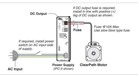
Power supply switching and fusing detail
