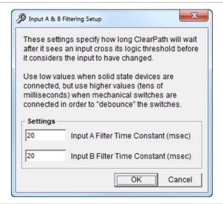
Input Filtering Setup
