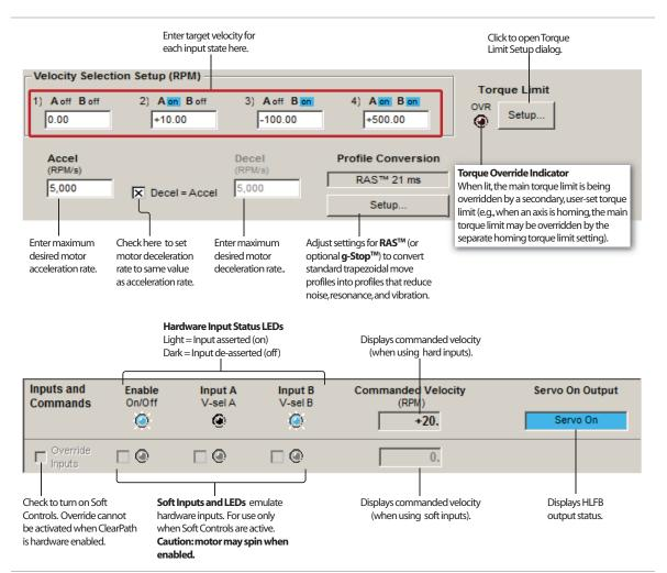
Mode Controls for mode "Ramp Up/Down to Selected Velocity"
