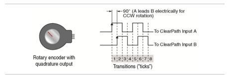
Example: Wiring a Mechanical Quadrature Output Device to ClearPath
