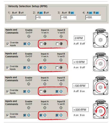
Change velocity and direction by checking Inputs A and B
