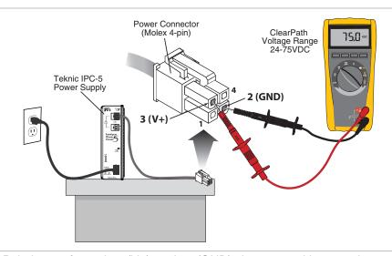
Polarity test from pin 3 (V+) to pin 2 (GND) shows a positive 75 volts
