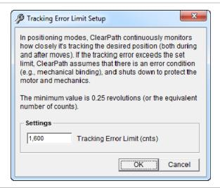
Tracking Error Limit Setup
