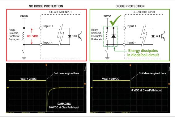
Use a flyback diode (right) to protect ClearPath inputs and outputs.
