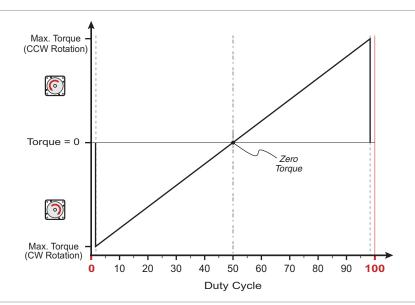
PWM duty cycle vs. motor torque
