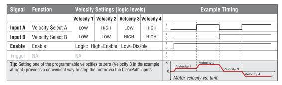
Ramp Up/Down to Selected Velocity Mode: Inputs and Timing Diagram
