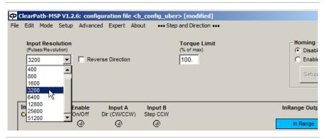
With the above Input Resolution setting, it takes 3200 step pulses to make this [800 count per rev.] motor rotate one full revolution.
