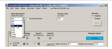
Using the above setting, 800 step pulses will make this [800 count] motor rotate one full revolution.
