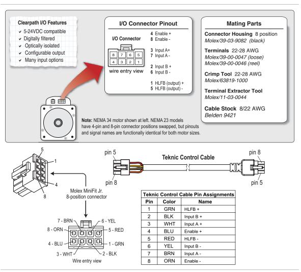
ClearPath I/O connector and mating parts
