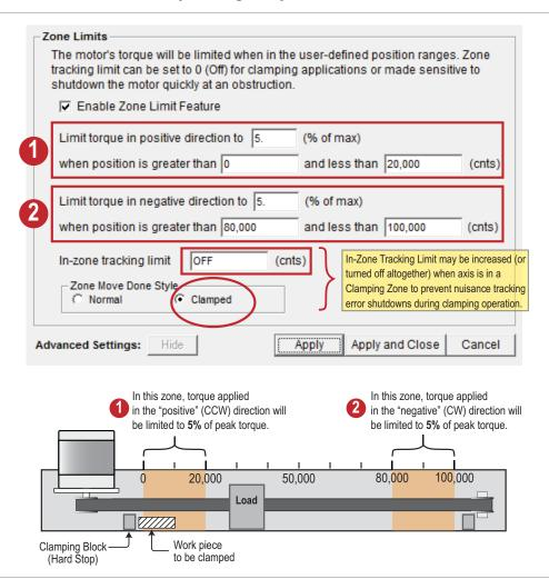
Zone Torque Limits (Clamped Move Done Style)
