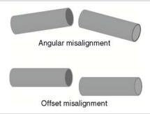
Some couplings are more forgiving of misalignment than others, but in general, misalignment will cause undesired vibration/noise, shortened bearing life, and even broken motor shafts.
