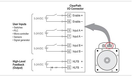
Simplified overview of ClearPath inputs and output
