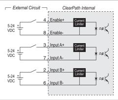
ClearPath Inputs shown with simple switches
