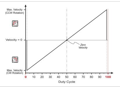
Graph of PWM duty cycle vs. motor velocity
